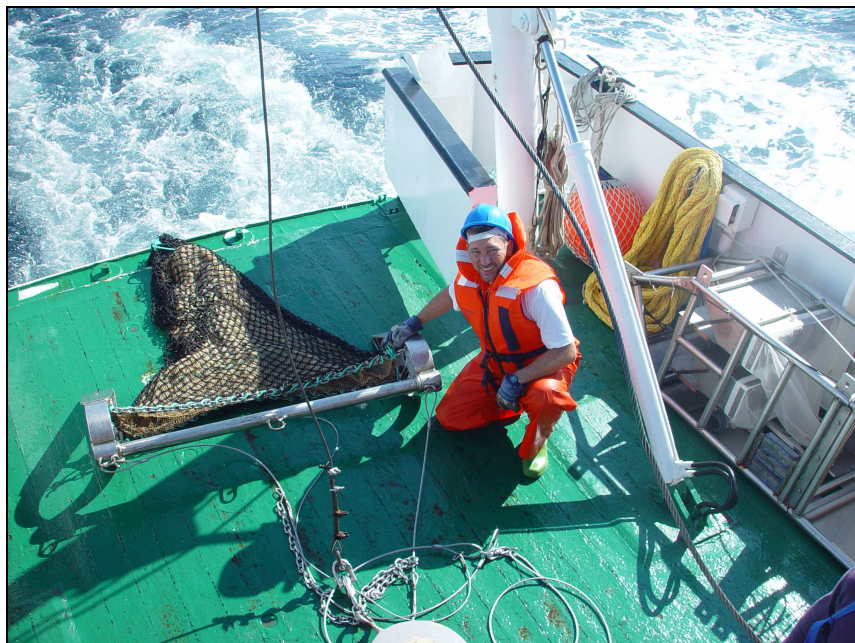
Fig. 5: The Agassiz Trawl employed during the expedition "DIVA-Artabria 1" on board of B.O. "Mytilus", F.J. CRISTÓBO photo.
