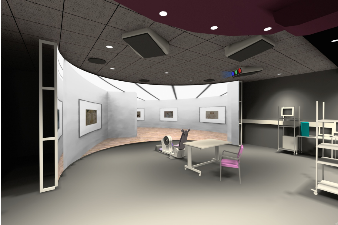
Figure 17: Schematic of PanoLab. The cylindrical screen with 3.5m radius shows a 220^\circ \times 50^\circ panoramic view using three projectors. Observers have an undistorted view of the projected image from the centre of the cylinder.
