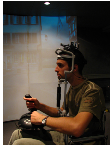
Figure 18: Left: Participant sitting on the wheelchair and viewing the street in Virtual Tübingen on the panoramic projection screen. The wheelchair is put on a podest so that the participants eyes were at the height of the screens centre. The physical and simulated FOV were matched to be identical at 220^\circ \times 50^\circ . Participants sat at a distance of 3 metres away from the screen. The wheelchairs wheels were tightened by expanders to allow only small physical motions of maximally 5cm in each direction. Right: Participant wearing the accelometer on the head, with the headposition stabilised on a headrest. Participants used a joystick to give vection ratings. Walkman-headphones playing sound of flowing water were used to mask external noise.
