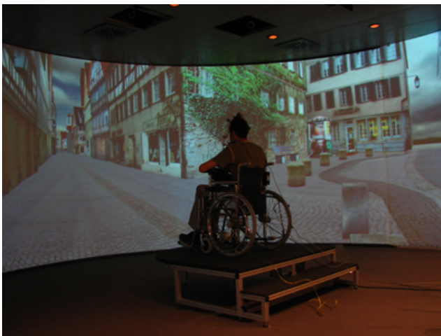
Figure 18: Left: Participant sitting on the wheelchair and viewing the street in Virtual Tübingen on the panoramic projection screen. The wheelchair is put on a podest so that the participants eyes were at the height of the screens centre. The physical and simulated FOV were matched to be identical at 220^\circ \times 50^\circ . Participants sat at a distance of 3 metres away from the screen. The wheelchairs wheels were tightened by expanders to allow only small physical motions of maximally 5cm in each direction. Right: Participant wearing the accelometer on the head, with the headposition stabilised on a headrest. Participants used a joystick to give vection ratings. Walkman-headphones playing sound of flowing water were used to mask external noise.
