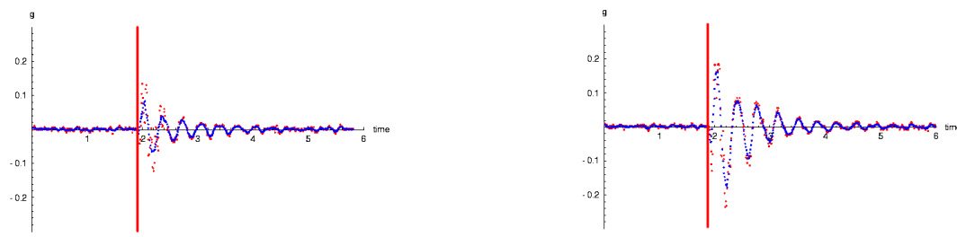
Figure 15: Physical acceleration profiles, recorded using an accelerometer attached to a participant's head. The left profile shows the 1 cm platform travel condition and the right one the 3 cm platform travel condition. The vertical red line shows the point at which the motion started.
