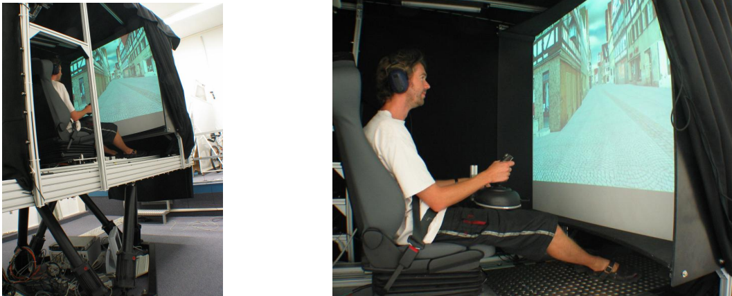
Figure 14: Participant seated on motion platform viewing the optic flow stimulus that was created using the Virtual Tübingen model. Participants wore active noise-cancellation headphones and used a Microsoft Force-Feedback Joystick to give the vection responses. During the experiment, the curtains were closed and lights were switched off.
