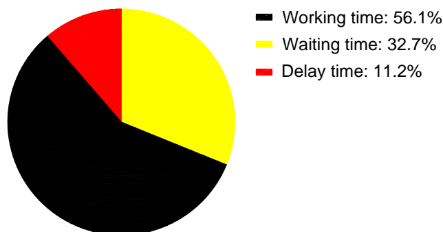
Figure 7.9: Utilization of MTBM (as % of total time) considering disturbances in project BV Recklinghausen V.8
