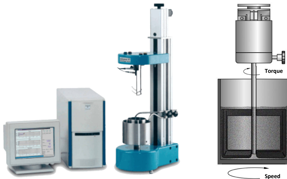
Figure 7-10: Schleibinger Viskomat NT (left) and working principle (SCHLEIBINGER GERÄTE TEUBERT U. GREIM GMBH (2012b))
