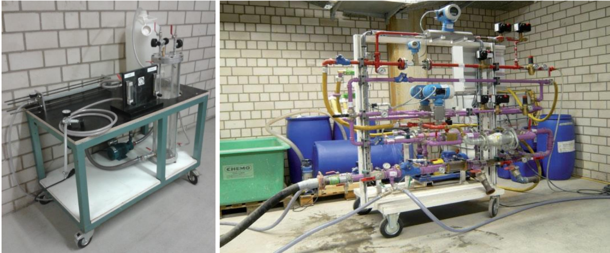
Figure 4-3: Foam generator 1 (“TLB mini foam generator”; left), Foam generator 2 (“TLB Laboratory Foam Generator”; equipped on real-scale foam generator) (THEWES & BUDACH (2010b))
