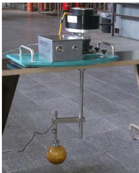
Figure 3-20: RheoCT: Prototype of a large-scale ball measuring system for rheological in-mixer measurements (FLEISCHMANN (2013))
