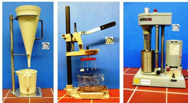
Figure 3-12: Recommended test methods determining flow properties of bentonite slurries: Marsh cone (left), ball harp (middle) and FANN rotational viscometer Model 35a.
