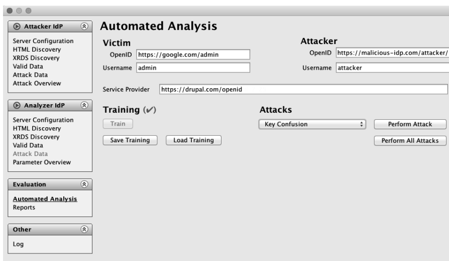
Figure 3.7: OpenID Attacker supports fully automated analysis. To use it, one has first to configure the victim's and the attacker's accounts, and then select the attacks to be executed.
