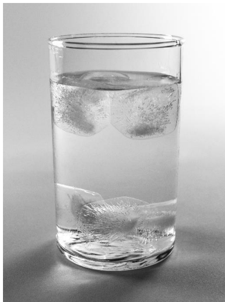
Figure 2.1 Heavy- and ordinary-water ice cubes in an ordinary water sample. The photograph was taken by Tietz 3 in the laboratories of Ruhr-Universität Bochum.
