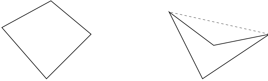
Figure 1.1: A convex quadrilateral (on the left side) and a reentrant quadrilateral (on the right). Note that, in the latter case, one of the four vertices of the quadrilateral falls inside the convex hull of the other three, as highlighted by the dashed segment.
