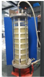
Figure A-3-4: Detailed view on the components of set-up for the testing of deep slurry penetration – Case B
