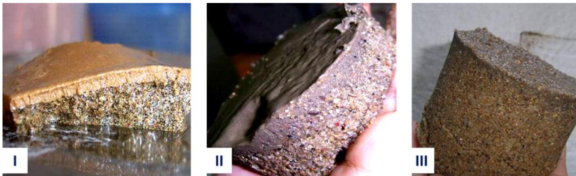
Figure 3-17: Experimental visualization of theoretically possible cases of slurry soil interaction (Min et al., 2013), Type I: filter cake – all grains of slurry are lodged on the surface of soil, Type II: filter cake with an infiltrated zone - some grains of slurry are penetrated into the soil, Type III: infiltrated zone without filter cakes - all grains of the slurry are penetrated into the soil
