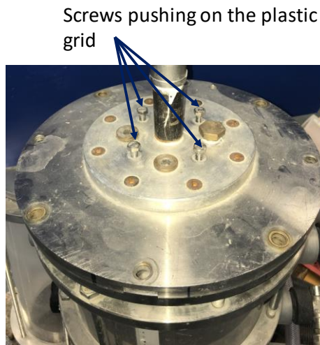
Figure A-3-6: Location of the screws at the cover of the soil cylinder
