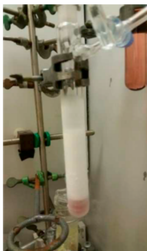
Figure 3. Crystallization of toluene adduct 4 shortly after removal of the cold bath.
