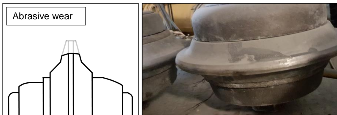
Figure 3-5: Wear pattern of abrasive wear of cutting discs.
