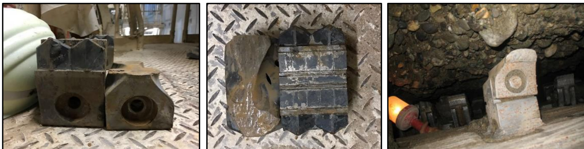
Figure 3-12: Worn ripper tools with different wear pattern (right picture: Köppl 2014, p. 109)
