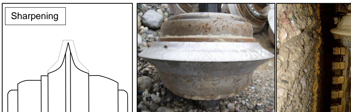
Figure 3-7: Wear pattern of sharpening of cutting discs (pictures from: (Köppl 2014, p. 93) and (Köhler et al. 2011)).
