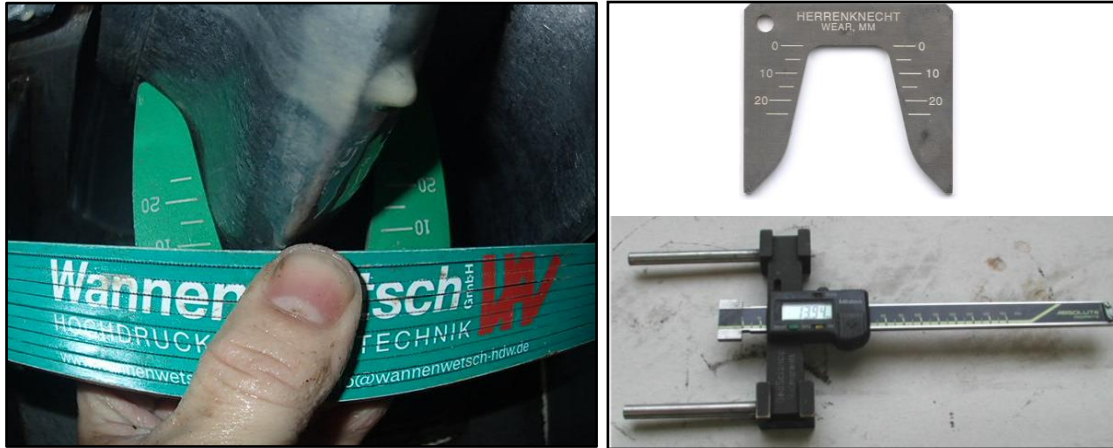
Figure 3-13: Wear measurement of cutting discs (pictures on the right side from Frenzel (2010, p. 56))
