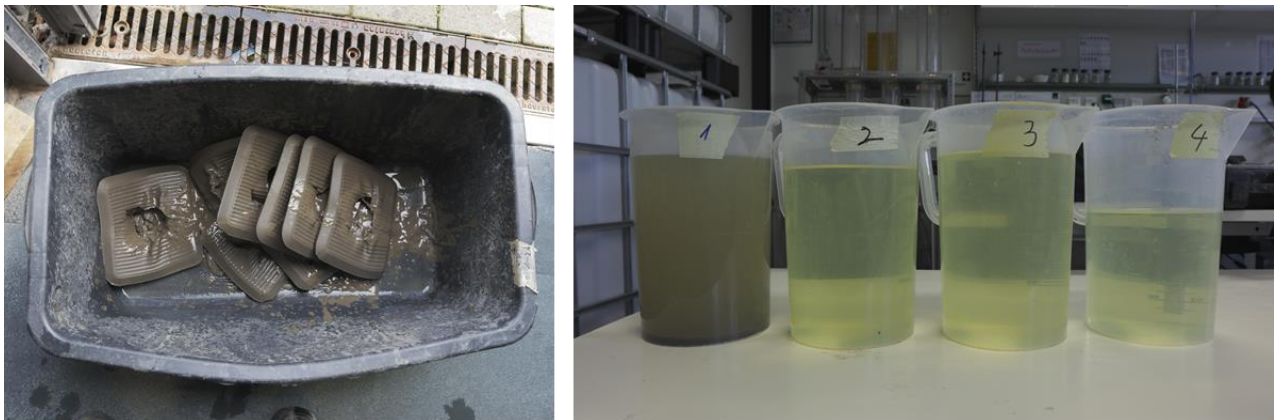
Figure 91: Filtration experiments with CUS: left) filter cakes, right) filtrate water
