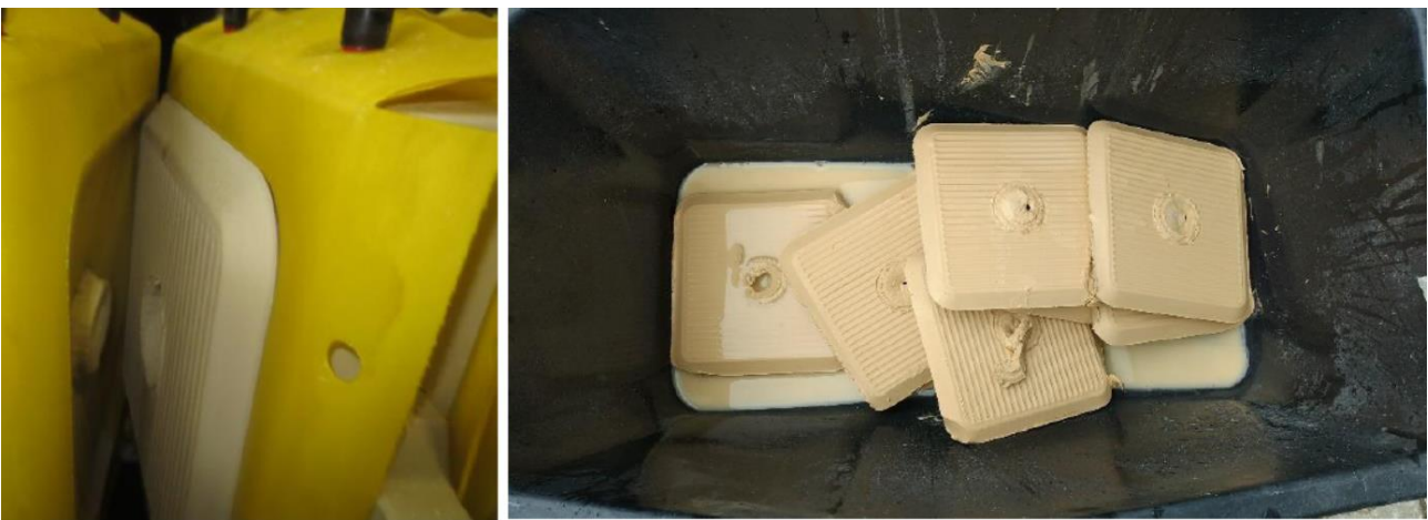
Figure 61: Filter cakes in the LCFP (links), released from the chambers (right)
