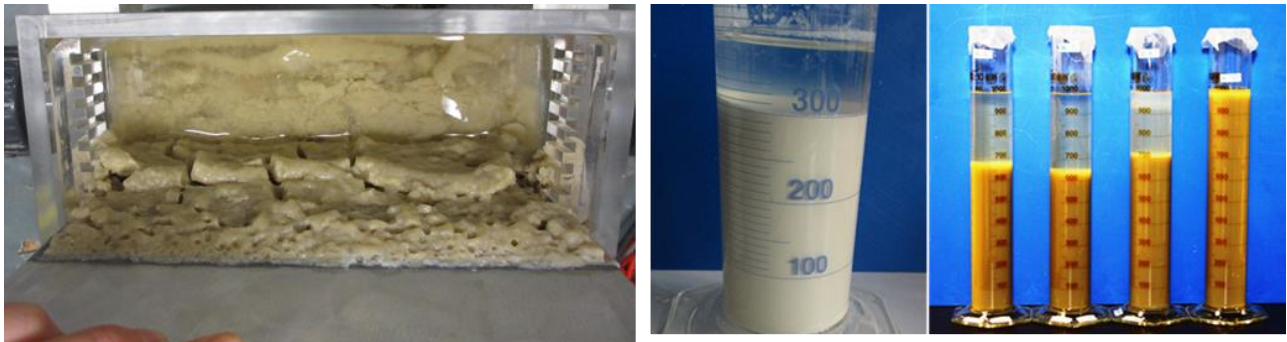
Figure 28: left: coagulated bentonite particles on the anode; right: destabilised remaining suspension (Popovic & Schöber, 2019)
