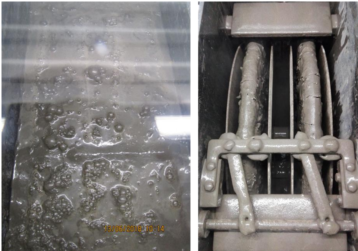
Figure 90: EC experiments with CUS: left) Gas bubbles during EC, right ) coagulated material on the anodes
