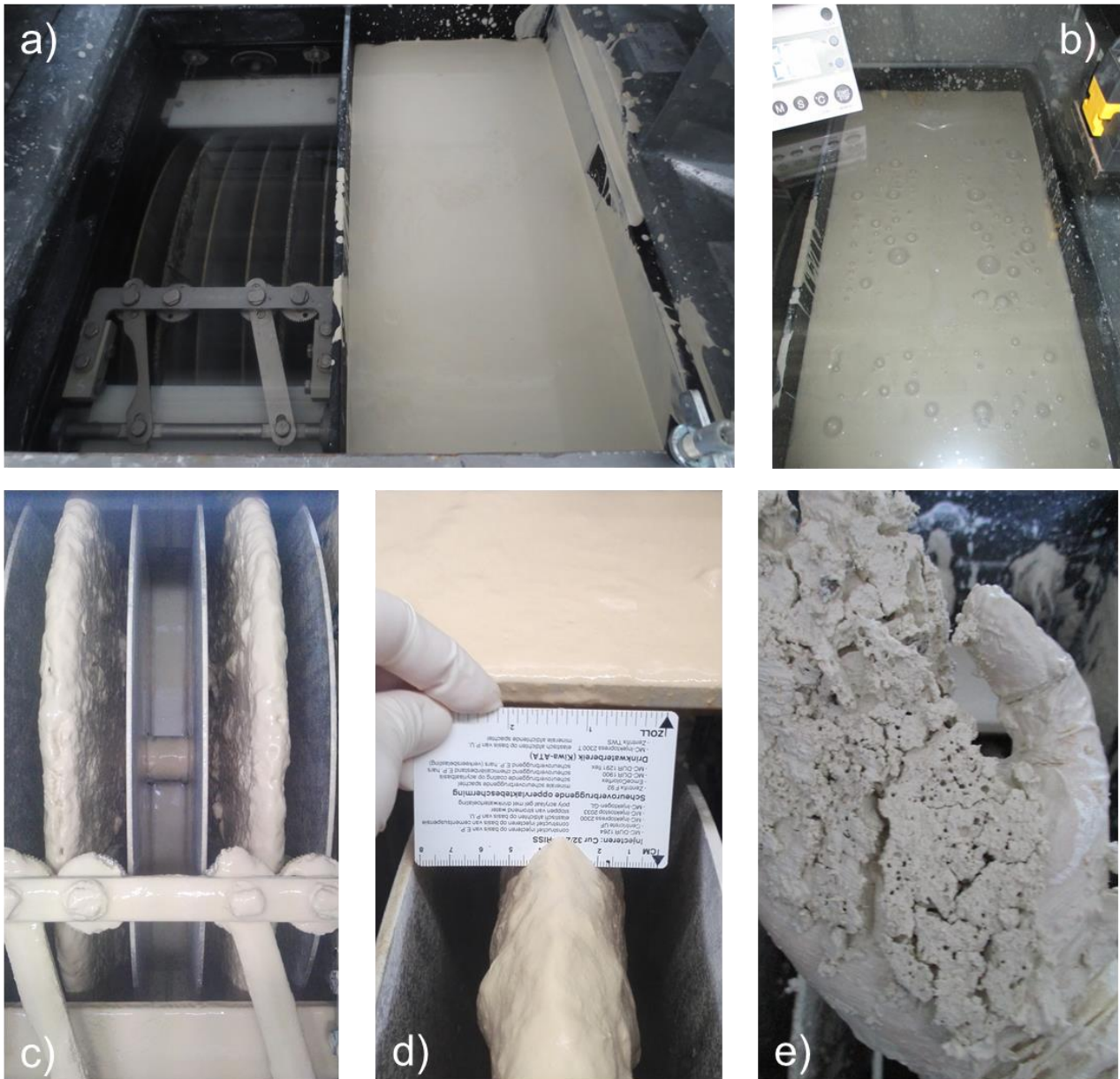
Figure 58: a) Before the experiment: water in the left chamber, SUS in the right chamber, b) Gas developing during the experiment c) After the experiment: the remaining suspension is pumped out of the cell, coagulated material remains on the anodes, d) Thickness of the coagulated material e) Coagulated material with small holes originating from oxygen development on the anodes
