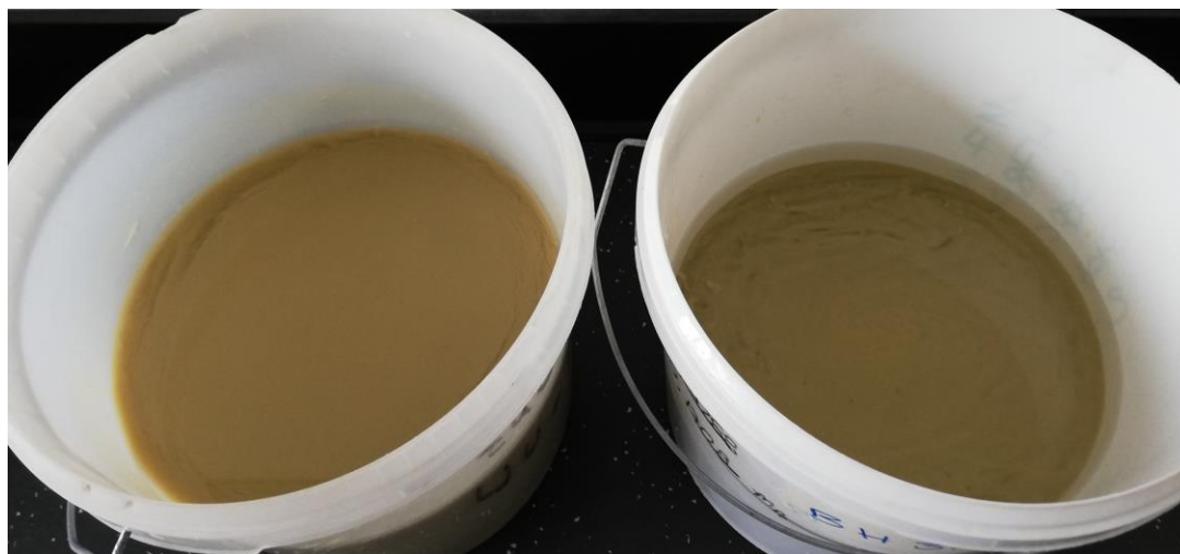
Figure 108: left) Fresh suspension mixed with tap water, right) Fresh suspension mixed with filtrate water after filtration with CA
