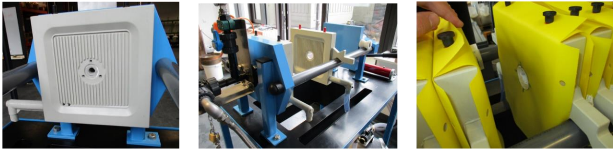
Figure 56: Openings in the centre of the chambers (Popovic & Schöber, 2019)
