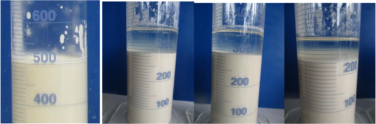
Figure 45: Sedimentation tests: a) no EC, b). R05, c) R10, d) R15, e) standard experiment
