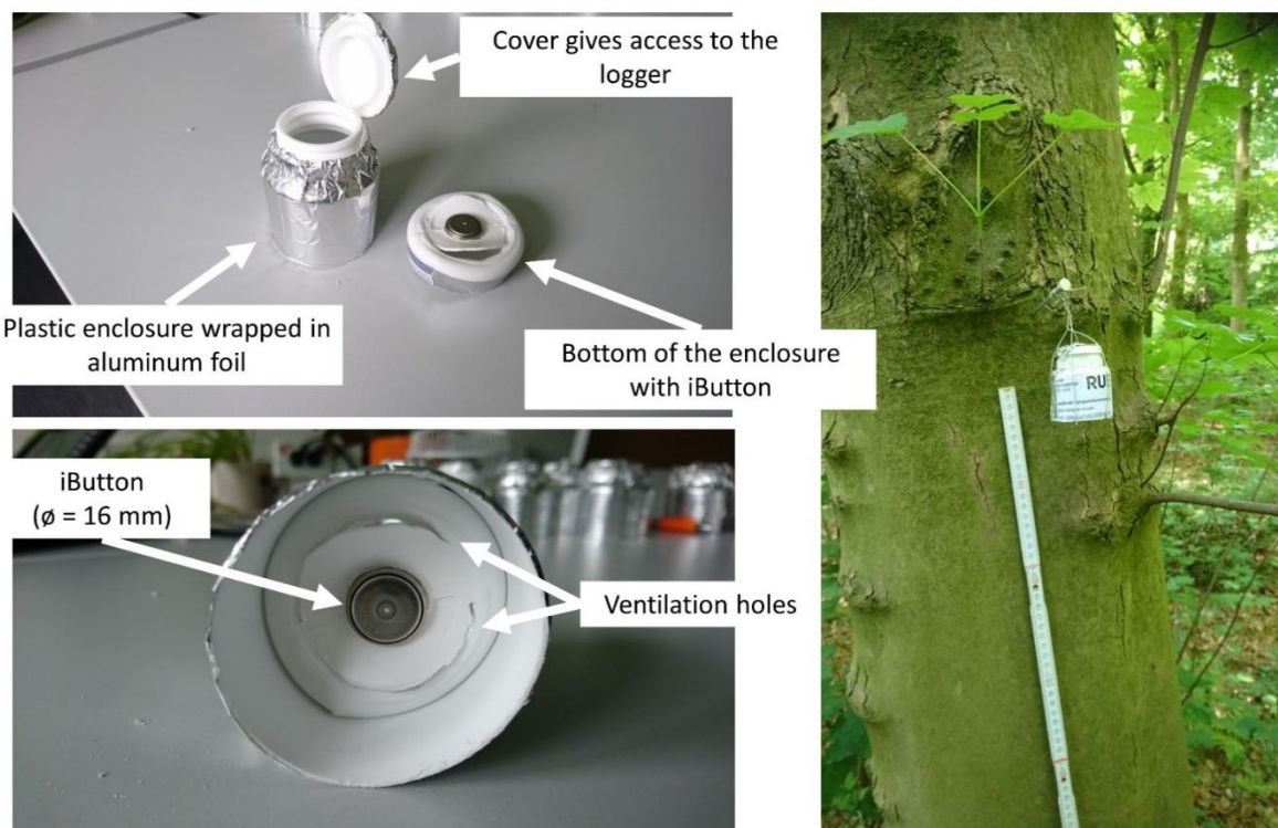
Figure 37: iButton with enclosure and example from installation.
