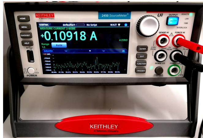
Figure 2.14: This figure shows a Keithley 2450 Source Measure Unit (SMU).
